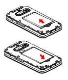
Unclip the cover, then remove the battery.
