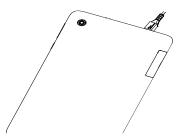
You are advised to fully charge the battery ( ). Charging status is indicated by a percentage displayed on screen. The percentage increases as the tablet is charged.
