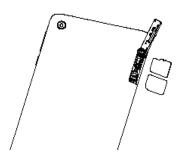
Your tablet only supports nano-SIM cards. Do not attempt to insert other SIM types like mini and micro cards; otherwise this may cause damage to your device.
